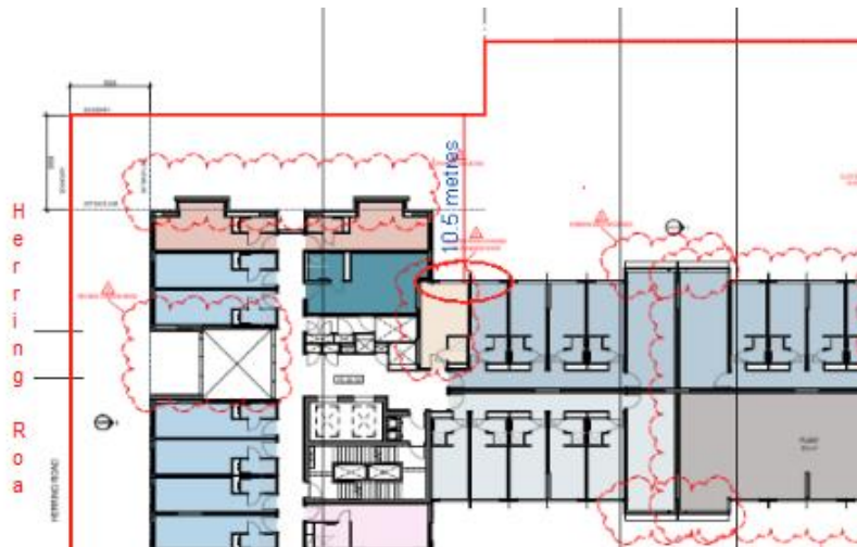
Figure 28 – Cluster room setback from 165 Herring Road. Source: Plan DA2012 8 - General Arrangement Plan Level 09 as prepared by AJC.
