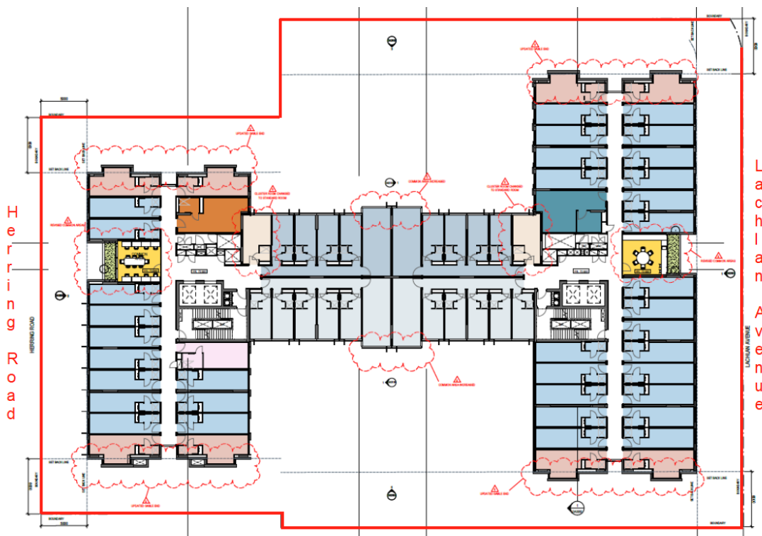
Figure 19 – Typical floor plan. Source: General Arrangement Plan Level 02 – DA2005 8. Note: Sky blue = Standard Studio. Orange = Large Studio. Pink = Premium Studio. Dark Blue = Accessible Studio. Dark & light grey (central spine) = Cluster rooms.
